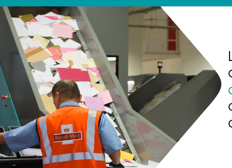
Letters are loaded onto a large conveyor belt which carries them up to a revolving drum.
